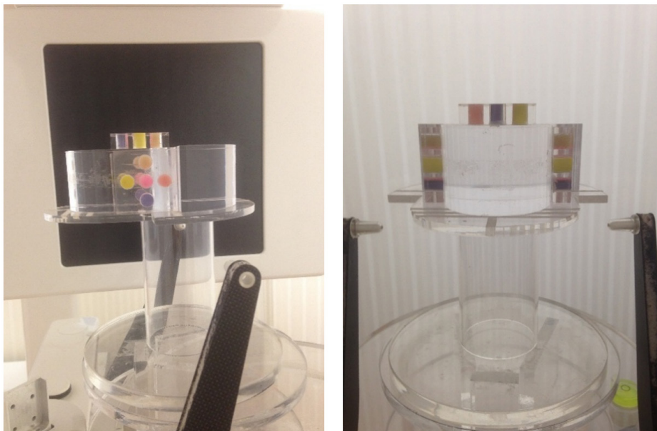
Fig. 4. The primary body of the phantom was positioned in a parallel alignment with the ground, with the ancillary instruments positioned at three distinct locations: on the left, right, and centre of primary body
