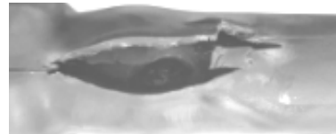
[Fig. 2] Insulation failure of damaged cable
