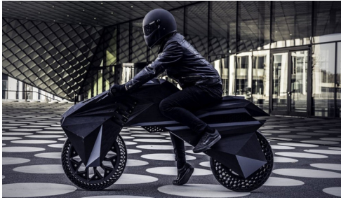
[Fig. 7] Redesigned e-bike with part consolidation [15]
