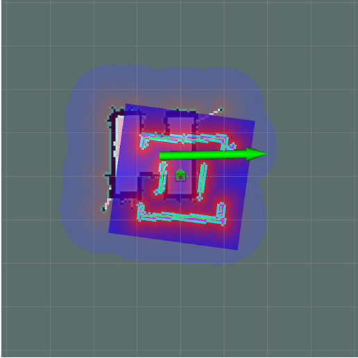
[Fig. 4] Adjustment of TurtleBot3's position through Estimation
