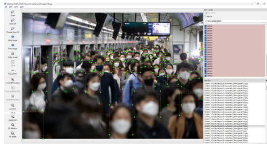
[Fig. 10] Labeling Work Using LabelImg
