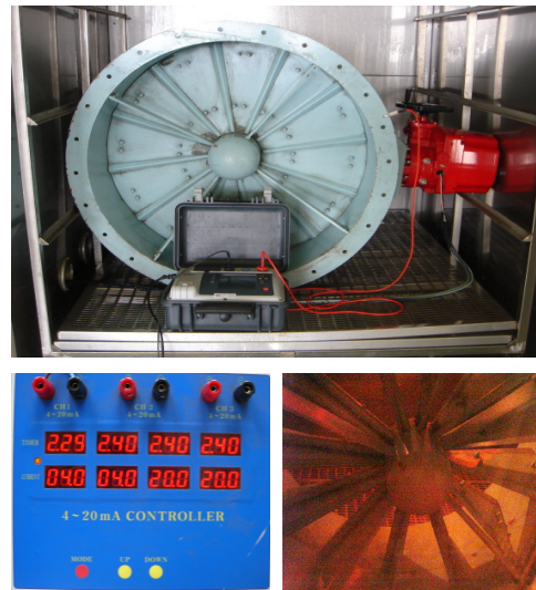
[Fig. 7] Environmental test apparatus for vane damper
