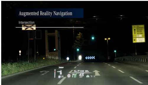
[Fig. 2] AR HUD Mounted on Vehicle
