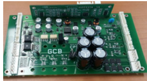
[Fig. 6] Generator Control Board
