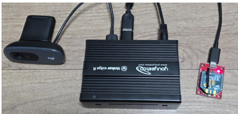
[Fig. 5] Web Camera connected to the ASUS Tinker Edge R edge device
