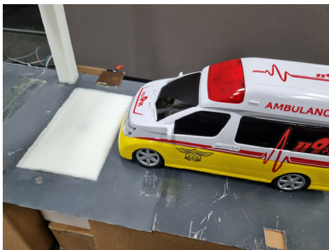
[Fig. 20] Automatic speed bumps for vehicles performing emergency duties
