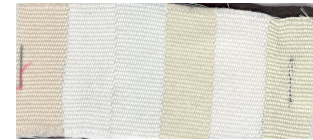
Wash fastness for the fabric cleared by Micro RC ® (Dye : Terasil WW Black o.w.f. 20%)
