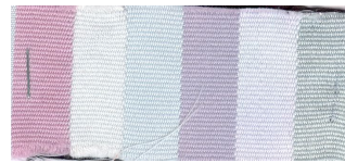
Wash fastness for the fabric cleared by a conventional R/C agent (NaOH/Na 2 S 2 O 4 )
