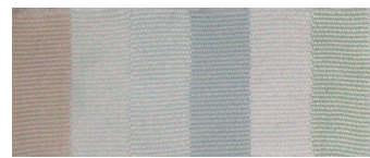
Wash fastness for fabric dyed at 110°C (Dye : Terasil WW Black o.w.f. 20%)
