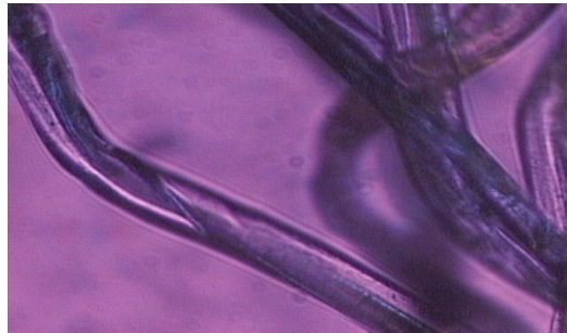
Fig. 13. Optical microscope photograph( 200) of acetate fiber used as tobacco filter.
