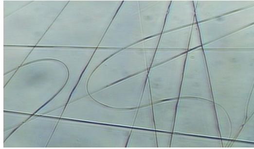
Fig. 12. Optical microscope photograph( 200) of acetate nano fiber prepared by electro-spinning.
