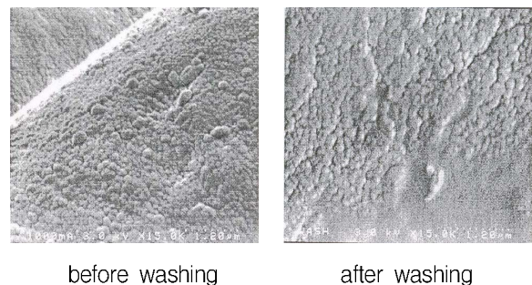
Fig. 10. SEM photographs of sputtered polyester fabrics before and after washing (X15,000). ( 3 \times 10^{-3} Torr of gas pressure and 6 cm of electrode distance, 1000 mA, 20 min)
