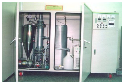
Fig. 3. Photographs of combination separation process system for dehydration purification of waste IPA solution.
