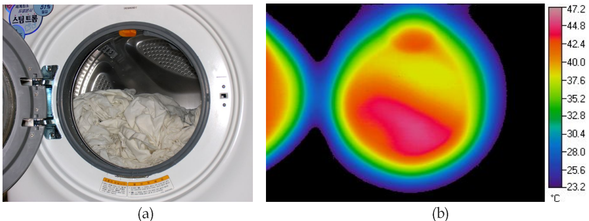
Fig. 6. Images of drum type test washing machine (a) Visible light image (b) Infrared light image after 15 minute steaming process.
