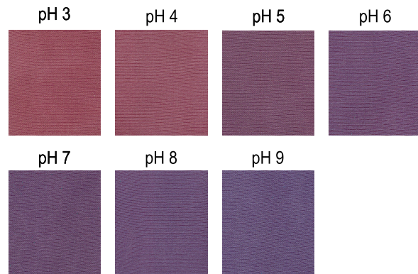
Fig. 6. Effect of pH on color of Gromwell-dyed silk fabric.(Dyeing condition ; temp. 60°C, time 30min., conc. 160%, o.w.f)
