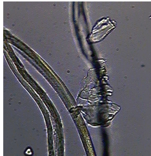
Fig. 7. Microscopic image of short fly and particles collected from the test.
