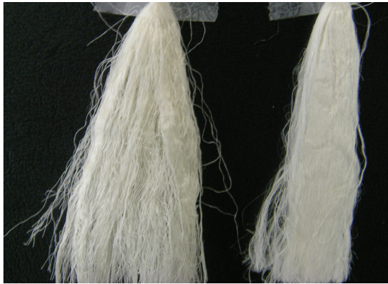
Fig. 4. Photograph of raw silk yarn bundles degummed at 80°C for 15 minutes(left) and 30 minutes(right) with 20%o.w.f. Marseilles soap.
