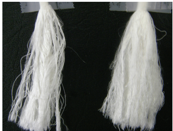
Fig. 7. Photograph of raw silk yarn bundles degummed at 80°C for 15 minutes(left) and 30 minutes(right) with 10%o.w.f. sodium carbonate.
