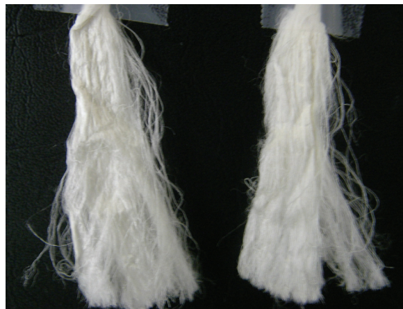
Fig. 6. Photograph of raw silk yarn bundles degummed at 80°C for 15 minutes(left) and 30 minutes(right) with 5%o.w.f. sodium carbonate.
