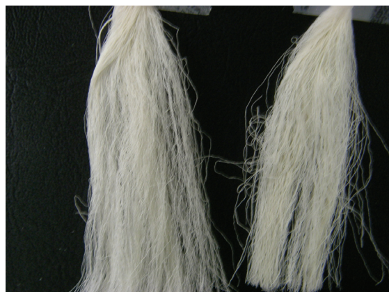
Fig. 3. Photograph of raw silk yarn bundles degummed at 80°C for 15 minutes(left) and 30 minutes(right) with 10%o.w.f. Marseilles soap.
