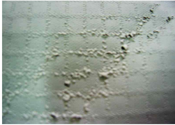
Fig. 2. Photograph of coat swelling on a film.
