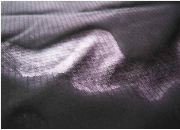
Fig. 1. Photograph of coat swelling on a fabric.
