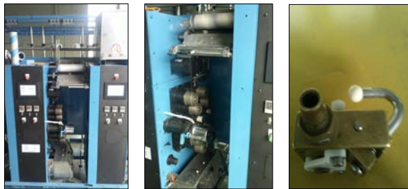
Figure 1. Air-jet texturing machine used in this study.
