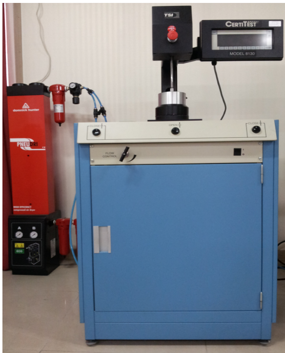
Figure 3. Photograph of TSI 8130 automated filter tester.
