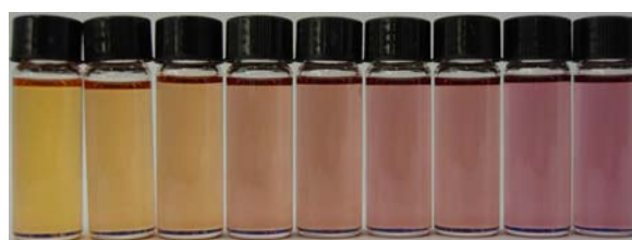
Figure 2. Photo images of color changes for chemosensor solutions with various guest anions in DMSO.
