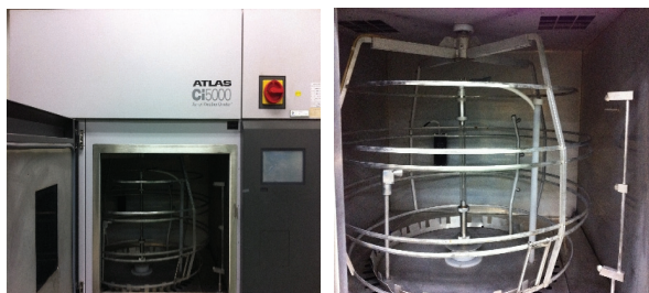
Figure 1. Weather resistance test(Xenon Arc Weather-Ometer Ci5000).
