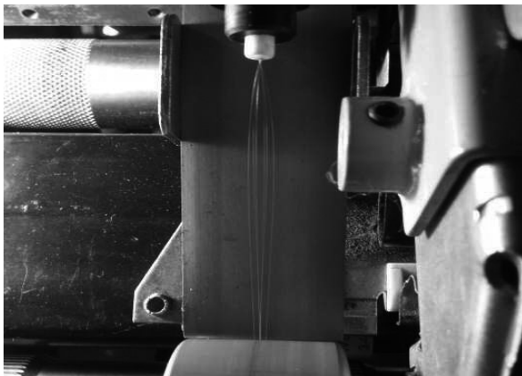
Figure 4. Multifilament separation of polyester filament on separation nozzle device in air blowing and electrostatic spinning(cyclone) frame.
