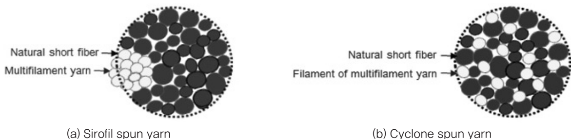
Figure 1. Cross section concept of sirofil spun blend yarn and cyclone spun blend yarn.
