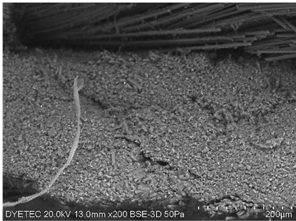
Figure 7. SEM image of the failure morphology of 3D braided composite tube.
