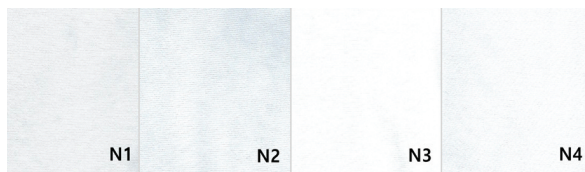
Figure 8. Adsorption color of 4 kinds of phthalocyanine NIR dye in 1% o.w.f. of polyester fiber.
