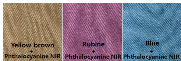
Figure 19. Phthalocyanine NIR dye and disperse dye dyeing on polyester fabric in the condition of using swelling agent.
