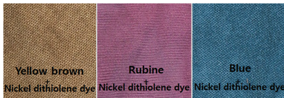
Figure 21. Nickel dithiolene dye and disperse dye dyeing on polyester fabric in the condition of using swelling agent.
