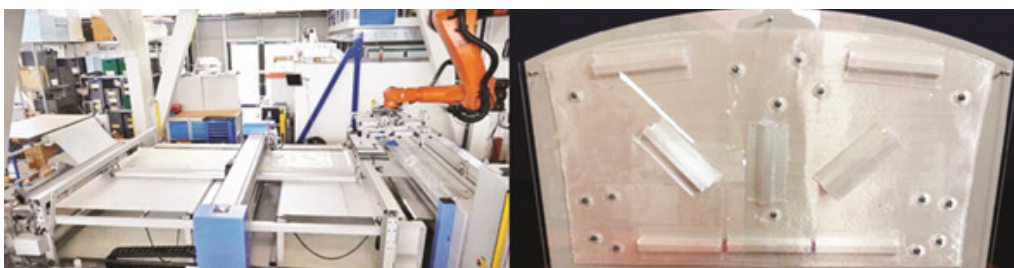
Figure 16. (a) Scheme of ITA preform auto manufacturing system. (b) ITA preform stitching unit and preform 24) .
