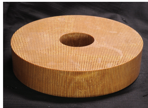
Figure 14. 3D woven composite for TPS, NASA 23) .
