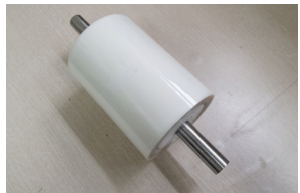
Figure 10. Scattering film roll coated by roll-to-roll process.
