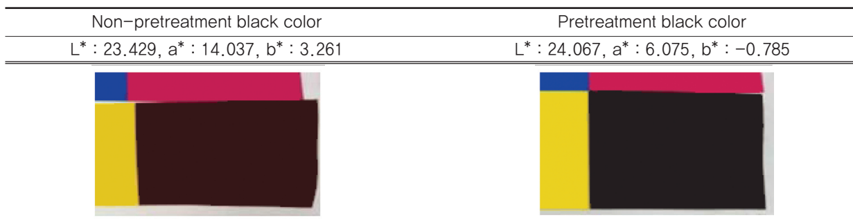
Figure 8. Comparison of black color of pre-treated nylon and non-treated nylon.
