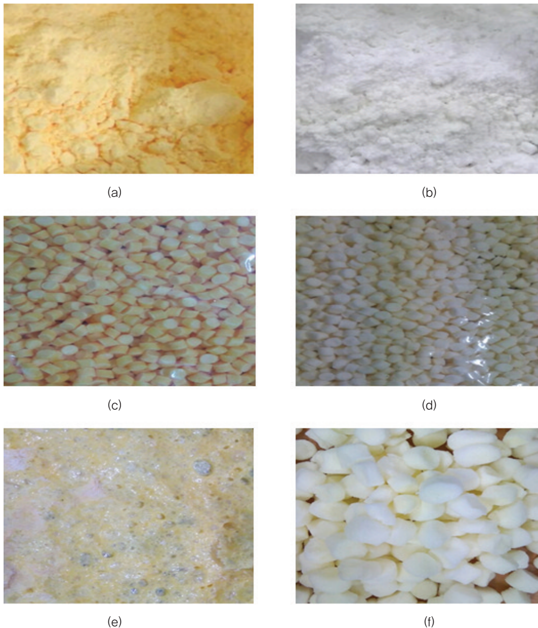
Figure 1. Images of ADCA chemical blowing agent of (a) powder, (c) master-batch chip, (e) after blowing procedure and images of thermally expandable microcapsule of (b) powder, (d) master-batch chip, (f) after blowing procedure, respectively.
