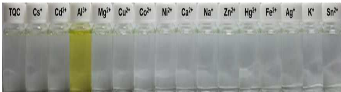
Figure 1. Color changes of TQC with various cations (10 \mu\text{M} ) in normal light.
