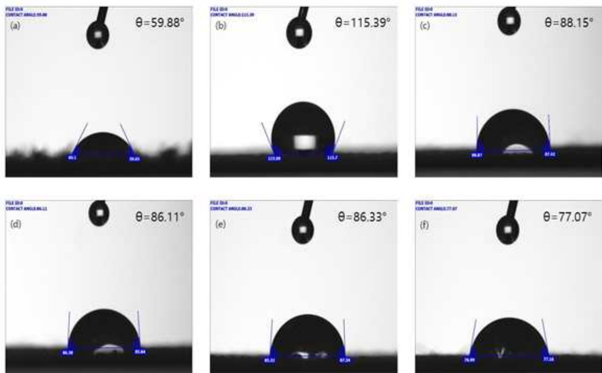
Figure 8. Contact angle of water droplets at 15% ODDMAC concentrations, curing(130°C, 10min) according to washing times; (a) untreated PET, (b) treated PET with 15% ODDMAC, (c) 5 times washing, (d) 10 times washing, (e) 25 times washing, (f) 50 times washing.
