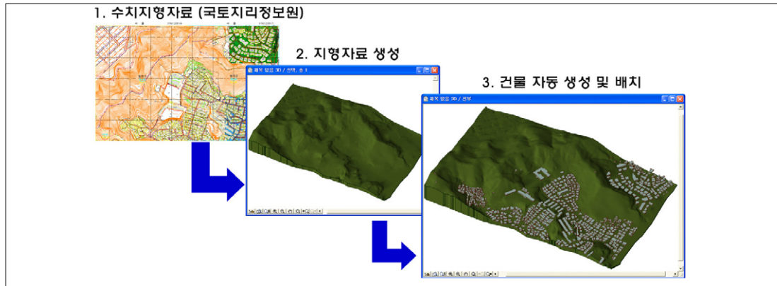
Fig. 2. Data processing steps of the input data processing system: Automated topographic data extraction and building placement from the digital topographic map, which is publicly available from the National Geographic Information System.
