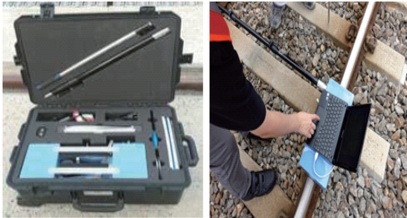
Figure 7. Rail roughness measurement system
