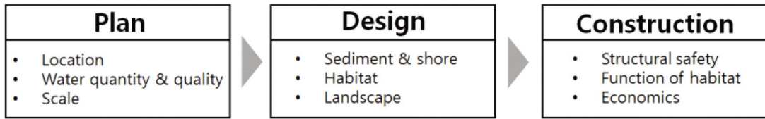
Figure 1. Overview of construction process for the ecological pond in this study.
