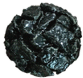
(c) Bio-stone ball coated with microorganisms
