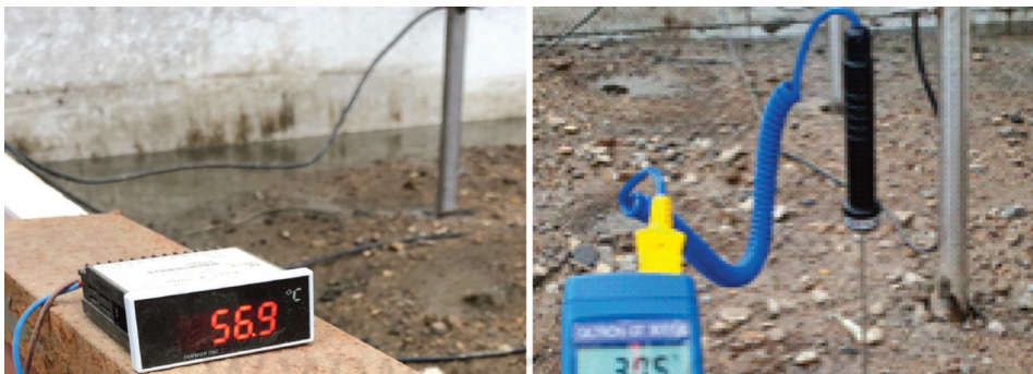
Figure 4. Monitoring of the electrode and soil temperature.
