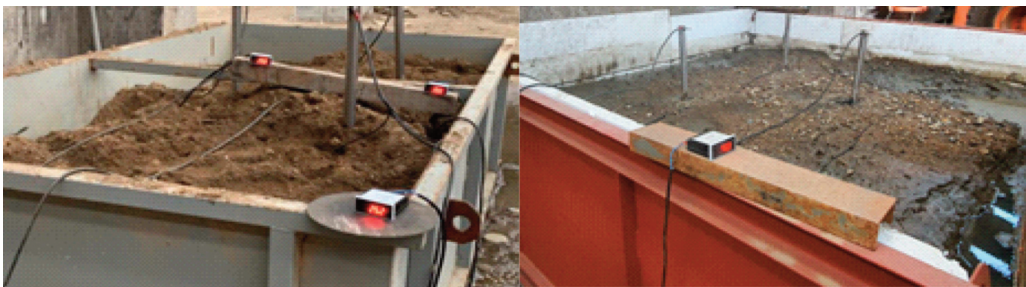
Figure 9. Pilot box experiment for evaluating heat transfer efficiency according to unsaturated (left) / saturated (right) soil conditions (Type: Pipe, Material: STS 316, Array: a triangular arrangement).
