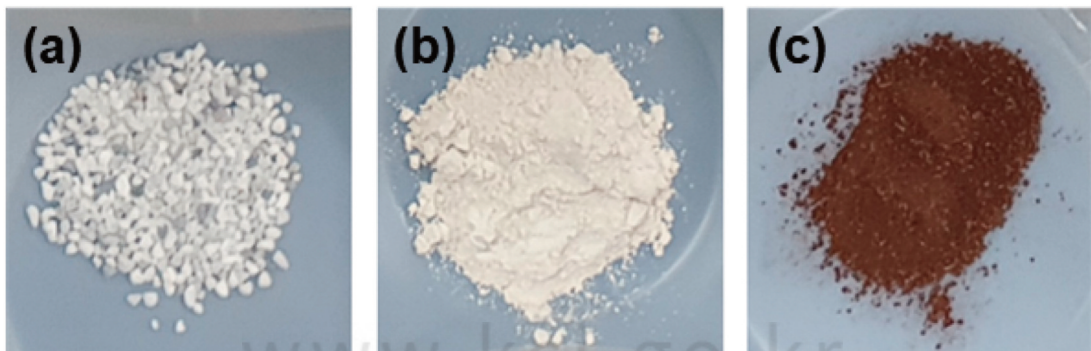
Figure 1. Commercial soil stabilizers employed in this study; (a) limestone, (b) AC-2, (c) Metafix.
