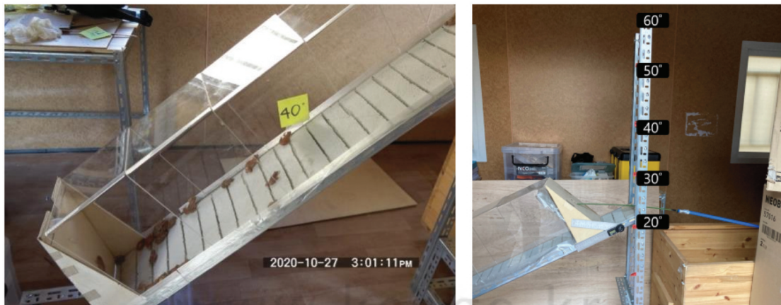
Figure 1. Experimental apparatus for frog behavior on concrete-product slope.
