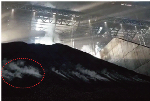
Figure 1. The spontaneous ignition of the indoor coal storage (Lee 2019).
