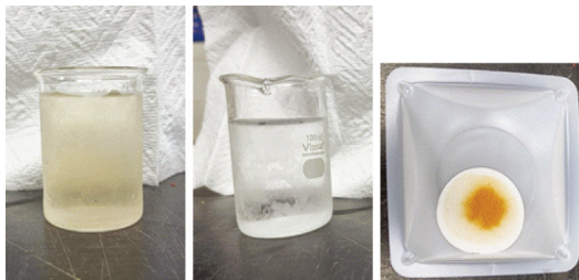
Figure 7. Results of water and filter paper after filtering SBS sample
